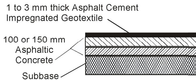
Figure 1 – Cross-section of asphalt concrete and fluid applied asphalt-geotextile barrier.
