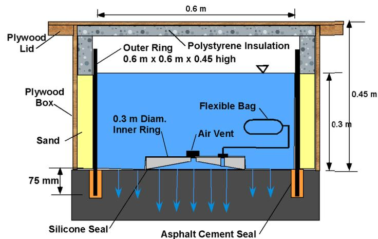
Figure 2 – Elevation view of sealed double-ring infiltrometer for measuring vertical infiltration into asphalt concrete barrier layer.
