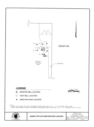
Following installation, a sufficient amount of an aqueous solution of hydrogen peroxide and catalyst was injected into each injection point. An injection flow rate consistent with litho logy for the site location was utilized. Two vent points were provided to prevent gas generated during the reaction from migrating away from the treatment zone. A soil vacuum extraction (SVE) blower was connected to the vent points to provide a sink, and recovered gas was treated with activated carbon.
