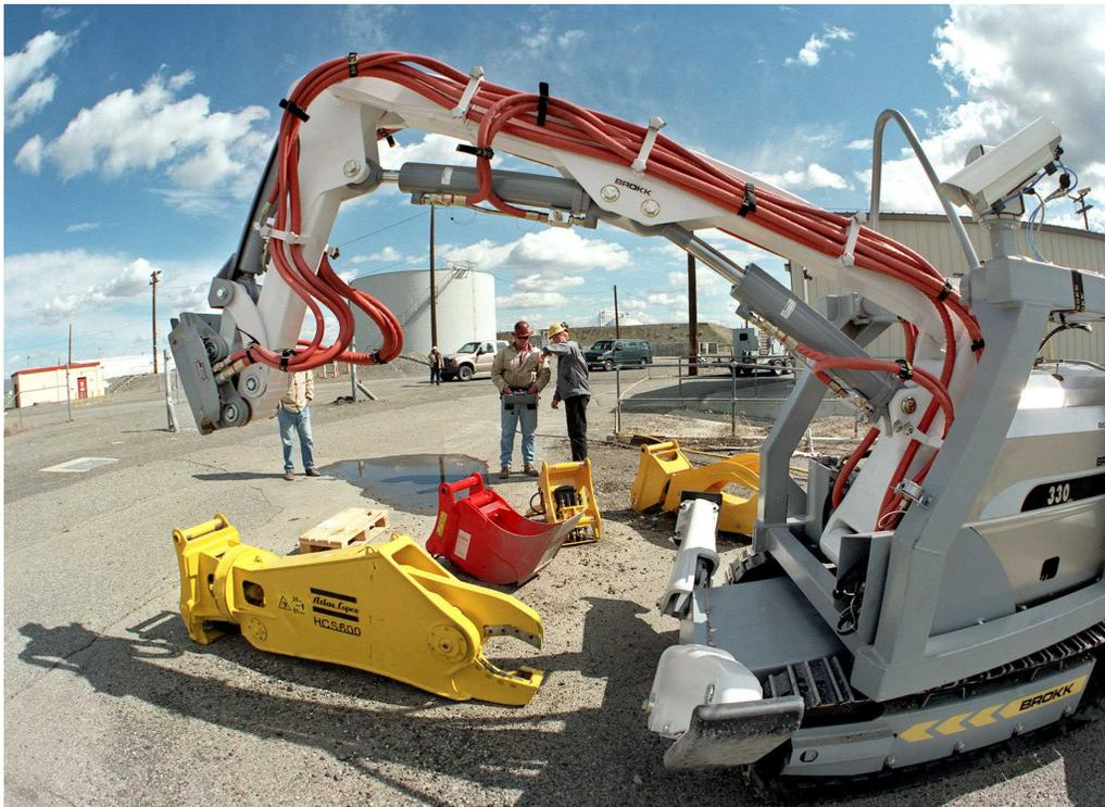
Figure 1 – Brokk 330N with multiple attachments
