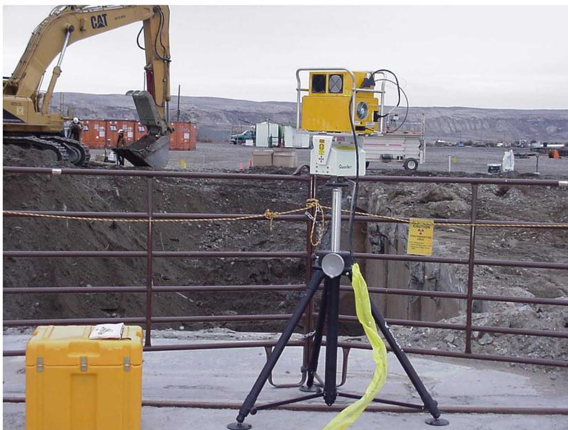
Figure 2 – Deployment of GammaCam at 105-F Reactor Fuel Storage Basin
