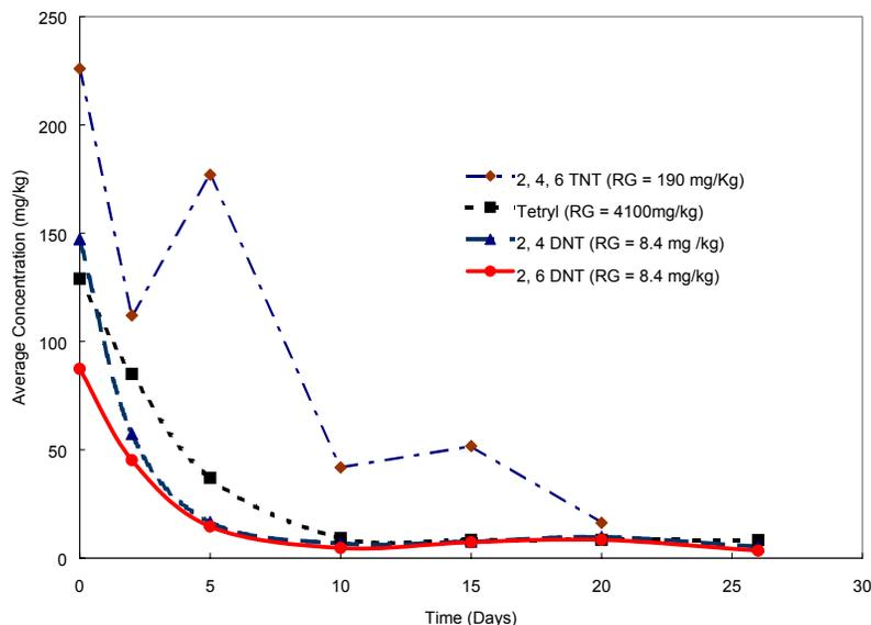
Figure 2. Change in Contaminant Concentration with days of operation obtained during field studies.
