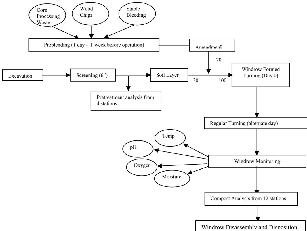
Figure 1. Process Flowsheet for Windrow Composting at JOAAP.
