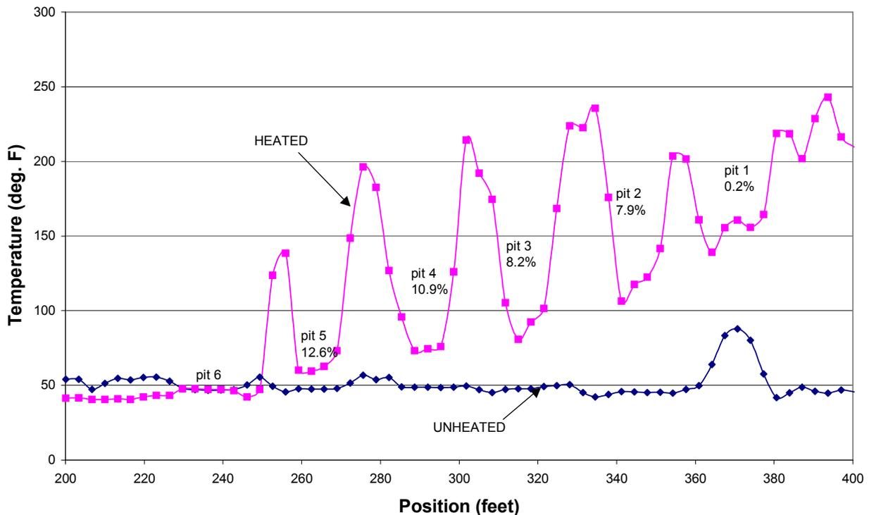
Figure 4: Temperature Rise Measured by DTS System in Heated Pits 1 through 5 (6 unheated), each with different moisture contents
