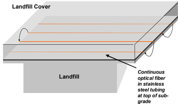
Figure 2: Continuous Fiber Optic Sensor Placed on Top of Landfill Subgrade
