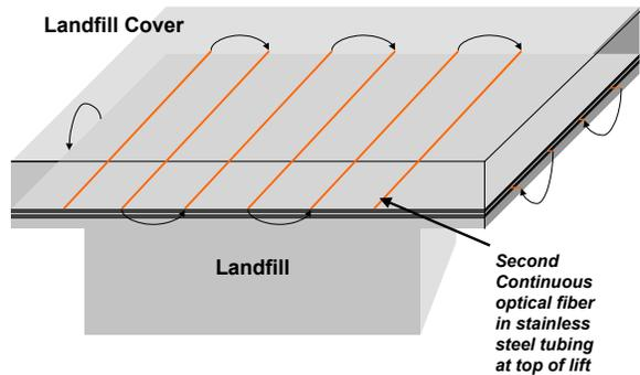
Figure 3: Continuous Fiber Optic Sensor Placed in Lift 30-40 cm above subgrade
