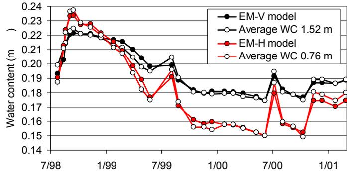
Figure 2. Monitored and predicted water content
