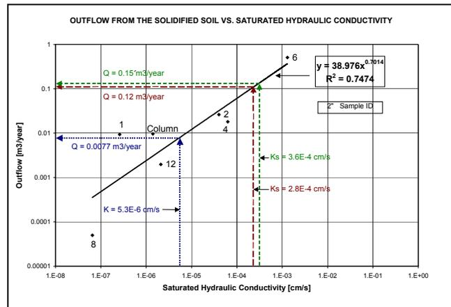
Figure 2 - Saturated Hydraulic Conductivity vs. Outflow.
