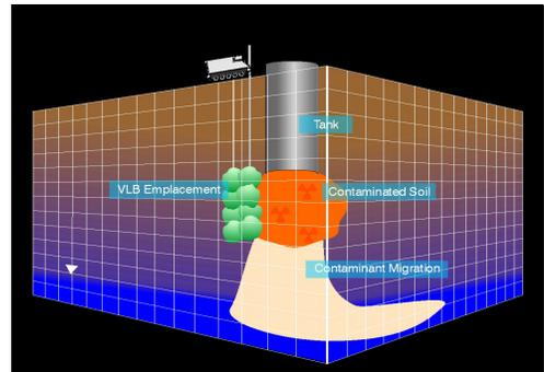
Figure 1 - Conceptual drawing of the BLIP Site.
