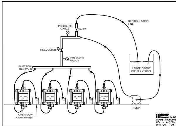
**Figure 1. Schematic of column injection apparatus.**
