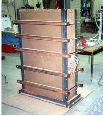
**Figure 1. Sand Tank Used for Laboratory Test Injections**
