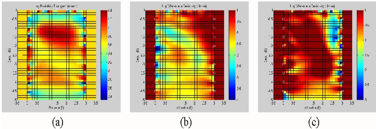
**Figure 2. ERT Results for the Pre-Injection (a), First Grout Injection (b), and the Second Grout Injection (c).**
