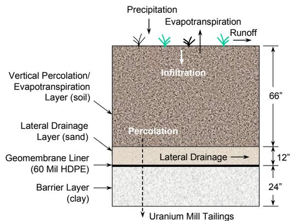
Figure 1. Conceptual model of percolation through the cover at the Monticello disposal site.
