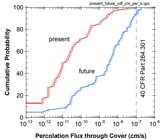
Figure 2. Cumulative probability plot of simulated percolation flux through the cover.
