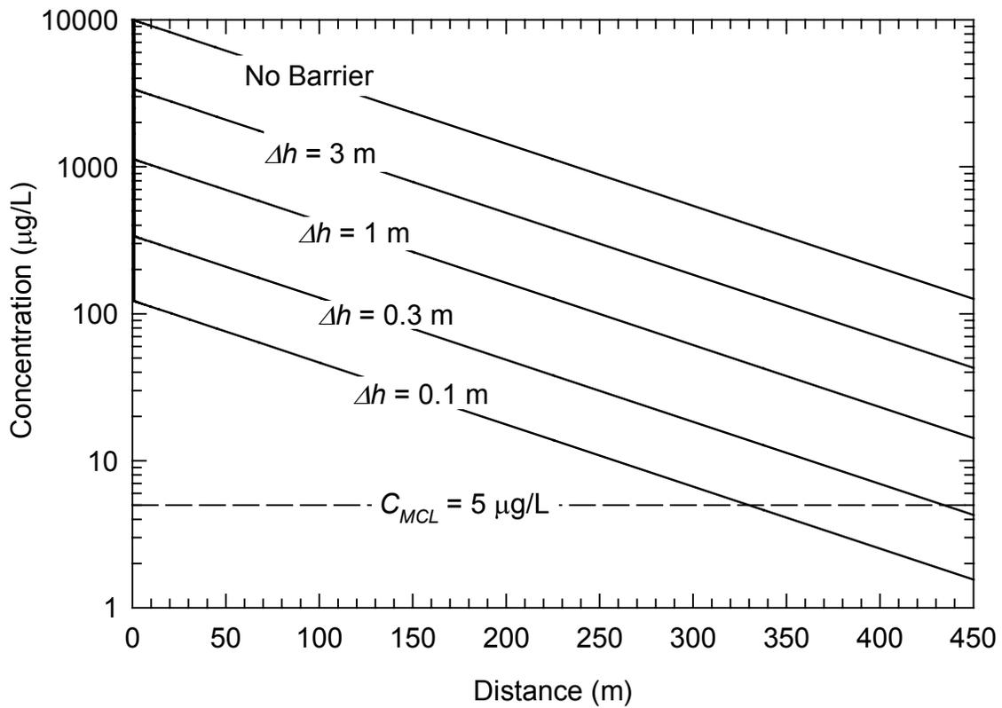
FIGURE 2. Benzene concentrations in the aquifer downgradient from the source area as a function of head difference across the barrier.
