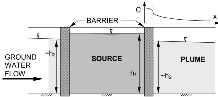
FIGURE 1. Cross-sections of barrier-controlled MNA near the source area.
