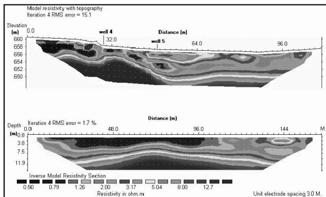
Figure 2. Examples of ground resistivity results. Darker shades are high resistivity zones.
