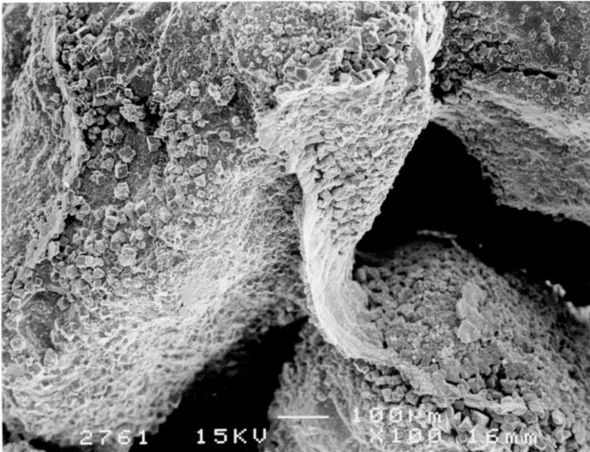
Figure 1 A Neutral Barrier: image from a Scanning Electron Microscope showing calcite layers over the surface of grains of quartz in unconsolidated sand. The calcite has formed continuous layers between adjacent sand grains, which lowers permeability without the need for complete pore filling.
