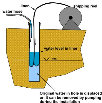
The Water FLUTE system uses an everting liner to transport a sampling and isolation system into the hole as shown in the drawing at the left. The liner is attached to the well casing and everted into the hole by “Just adding water”. The fifth photo (next page) shows the installation, from a large reel, of a 330 ft. system with 15 sampling intervals in a 6-inch diam. hole for the Univ. of Waterloo at Cambridge, Ontario. The entire installation took about 8
