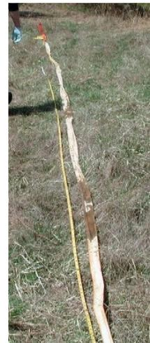
The massive staining seen in the 4th photo at about 20 ft and 30 ft in a 45 ft hole are the result of two thick layers of solvent intersected by the push rod at the same site as photo 3. The brown color is that of the solvent. The dye stains are on the fringes of the brown stains. This technique allows a positive location of the elusive DNAPL.
