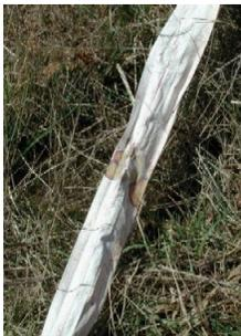
ft in a 45 ft hole are the result of two thick layers of solvent intersected by the push rod at the same site as photo 3. The brown color is that of the solvent. The dye stains are on the fringes of the brown stains. This technique allows a positive location of the elusive DNAPL.
