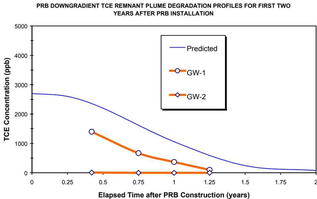
**FIGURE 1. PRB Downgradient Groundwater Monitoring Data.**
