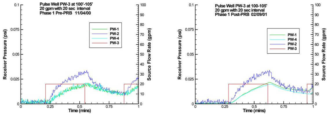
**FIGURE 2. Pre and Post PRB Construction Pulse Interference Tests.**
