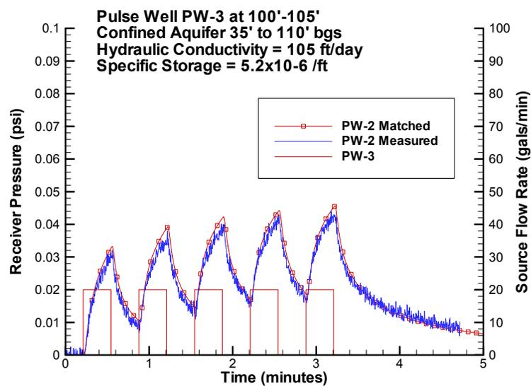
**FIGURE 1. Predicted/Matched and Measured Receiver Well Response.**
