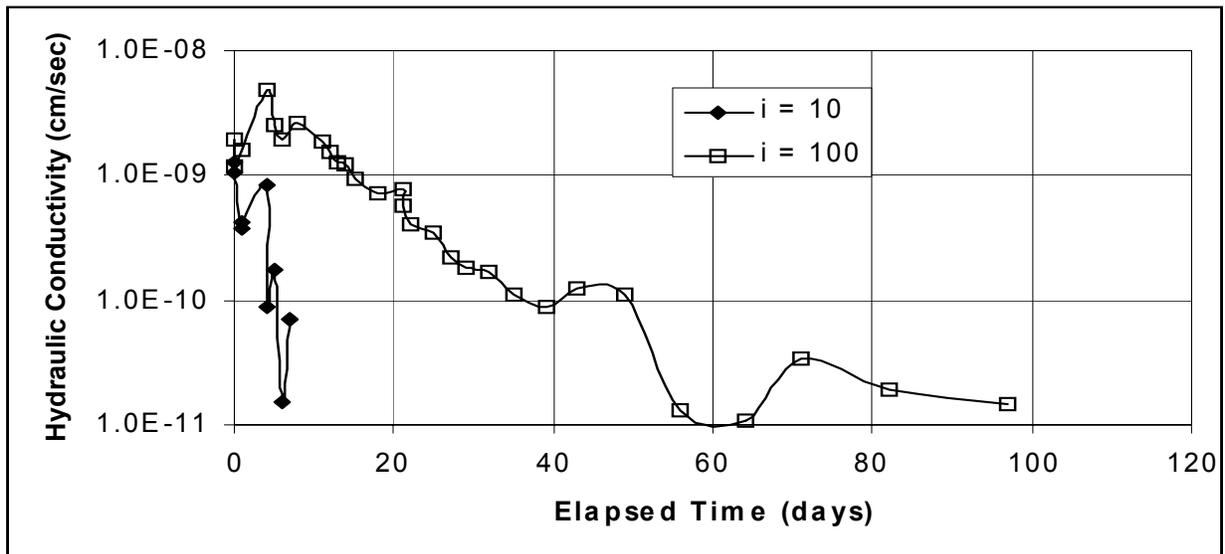
Figure 1 – Hydraulic Conductivity variations as a function of duration of permeation.
