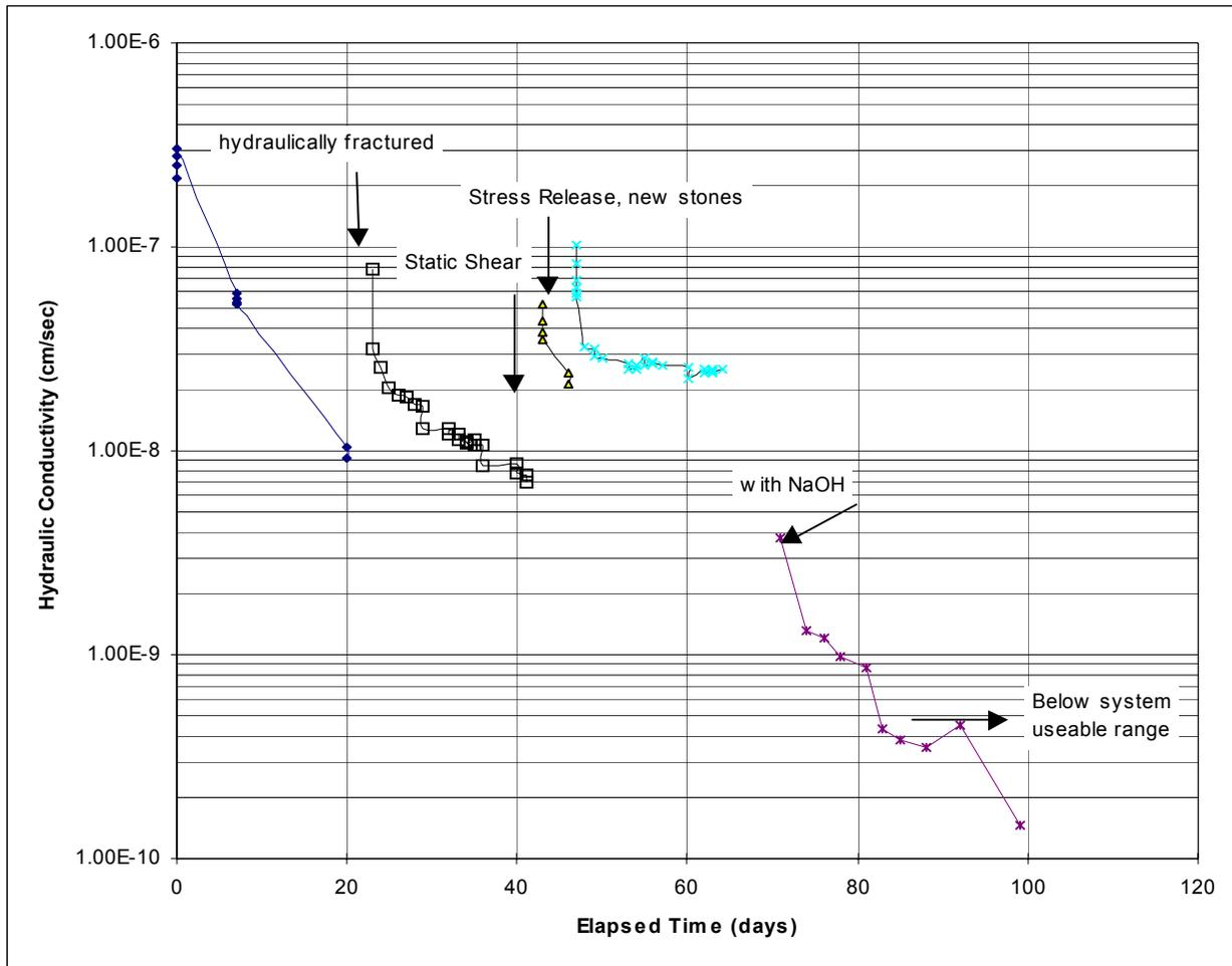
Figure 3 – Example of self-hardening slurry response to stressing and permeant pH
