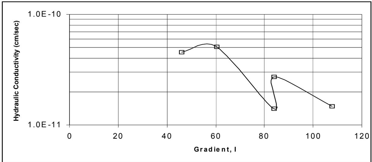
Figure 2 – Example results of hydraulic conductivity vs. gradient
