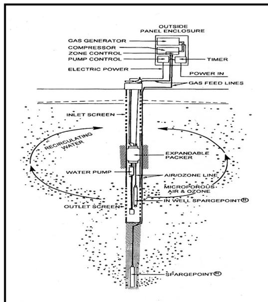
**Process Overview:** The ozone-sparging process involves the injection of air-encapsulated ozone into groundwater, to provide *in-situ* treatment. The sparging apparatus is designed to produce “micro-bubbles” sized at 0.05 mm (0.002 inches). This small air bubble size provides a high surface area to volume ratio to maximize treatment efficiency, and also allows the air/ozone gas to readily flow between soil pore spaces to attack the target compounds in groundwater (1).
