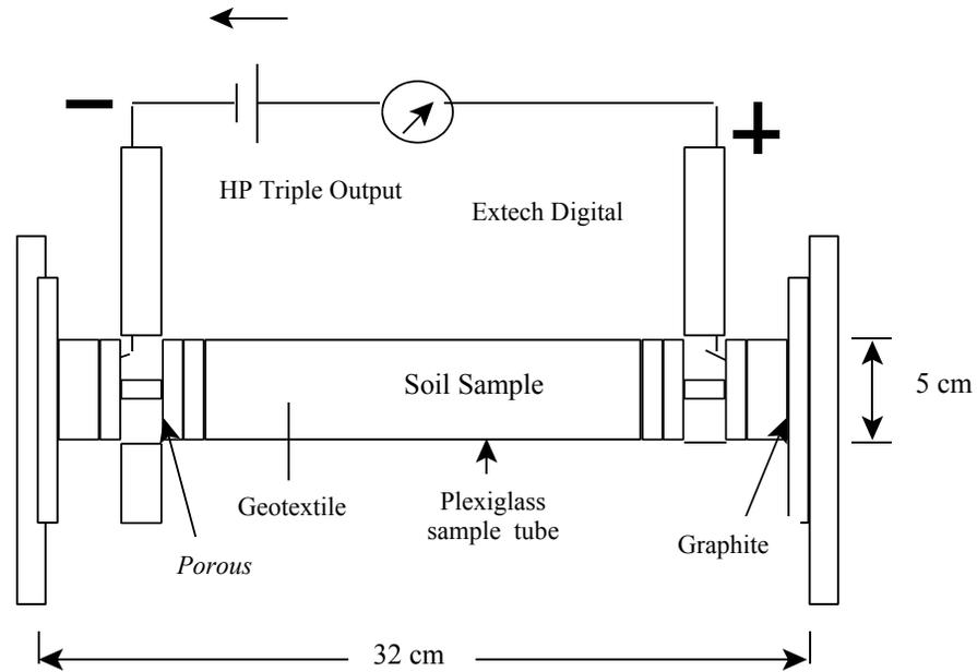
Figure. 1. The electro kinetic cell.
