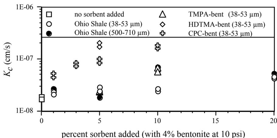
**Figure 2. Effects of Sorbent Addition on  $K_c$  (with 4% Bentonite at 10 psi)**
