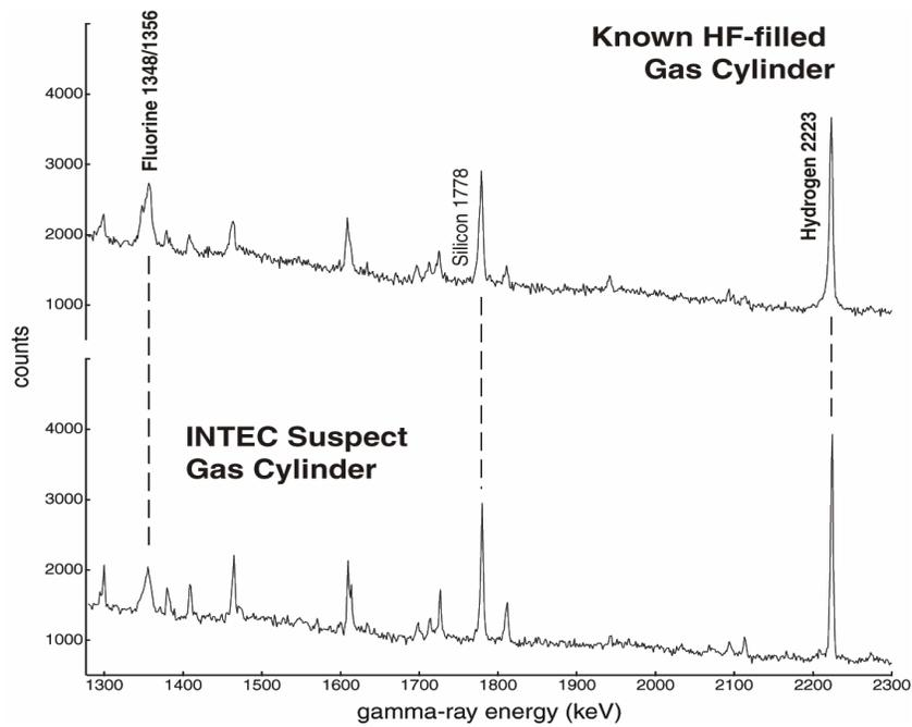
Figure 1. PINS spectra of HF cylinder.
