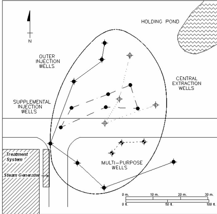
Figure 1. Site map and well-field layout for the SS/HPO demonstration at PORTS. The holding pond to the northeast is the source of the contamination. The TCE plume extends 1,900 ft to the east of the holding pond.
