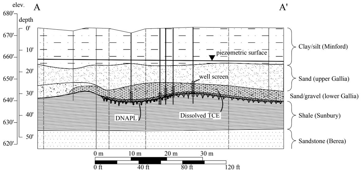
Figure 2. West-east cross-section through the demonstration area with the interpreted DNAPL distribution and location of example wells screened in the lower Gallia.
