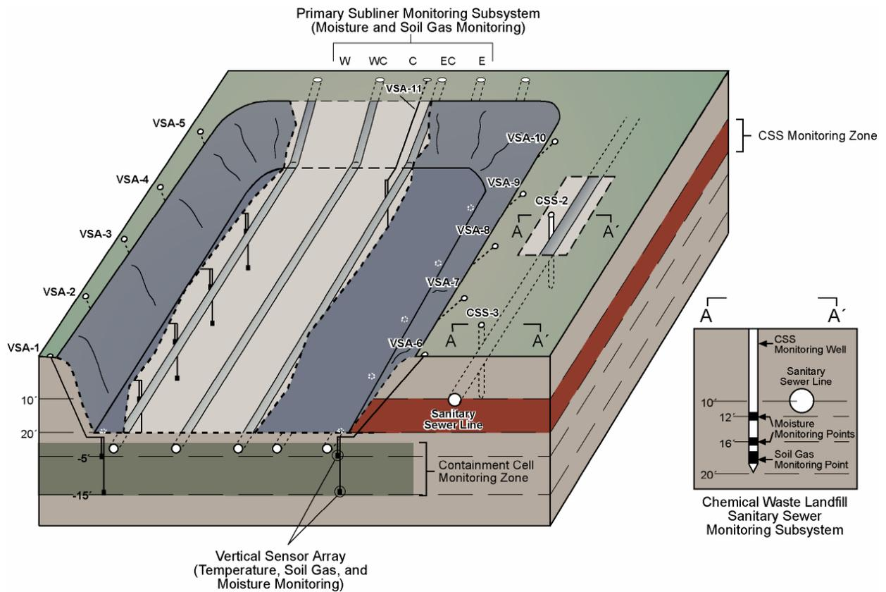
Figure 1 – Schematic Block Diagram Showing the Spatial Distribution of the Vadose Zone Monitoring Subsystems within and Adjacent to the CAMU Containment Cell.
