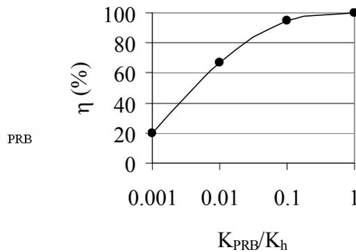
Figure 1b – Summary of the results for PRB hydraulic capture as a function of  $K_{PRB}/K_h$ .
