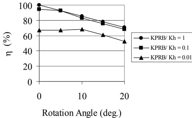
Figure 2a –Simulation results for  $\eta$  as a function of wall rotation angle.
