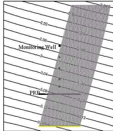
Figure 2b Simulation results for 15° shift in groundwater flow direction ( $K_{PRB}/K_h=1$ ).
