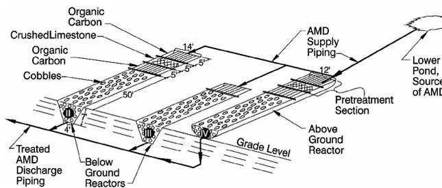
Figure 1. Layout of bioreactors.
