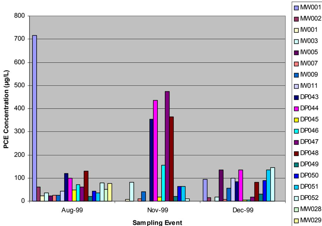
**Figure 1:** Results from the Pilot Test indicate the initial release of PCE from an adsorbed phase followed by chemical destruction via Fenton's reaction. Results shown are from the shallow zone and are typical for the site.
