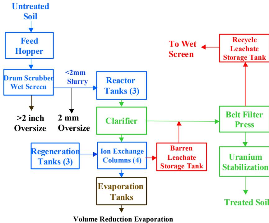
**Figure 1: Soil Washing Process Simplified Flow Diagram**
