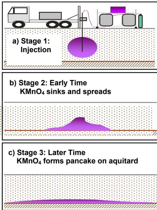
**Figure 1: Schematic of  $\text{KMnO}_4$  injection set-up, and conceptual model of  $\text{KMnO}_4$  distribution with time caused by density-driven advection.**
