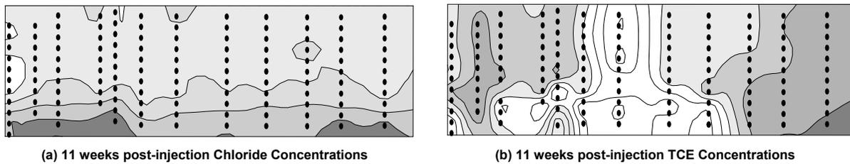
**Figure 4: 11-weeks post-injection a) Chloride and b) TCE concentrations, showing increased chloride concentrations to greater than 5000 mg/L at the aquitard interface, and decreased TCE concentrations to less than laboratory detection limit.**
