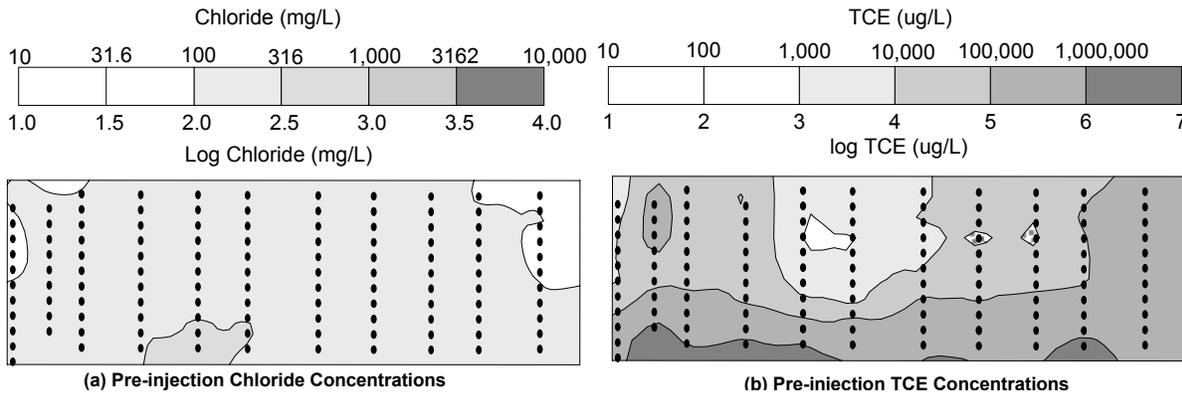
**Figure 3: Pre-injection a) Chloride and b) TCE concentrations, showing chloride generally less than 300 mg/L, and TCE concentrations greater than solubility at aquitard interface where DNAPL presence was also confirmed in 50 % of the cores.**
