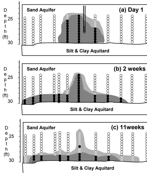
**Figure 2: Observed  $\text{KMnO}_4$  distribution with time. Light and dark shading indicates low and high concentrations of  $\text{KMnO}_4$ , respectively, based on colour with lab confirmation.**
