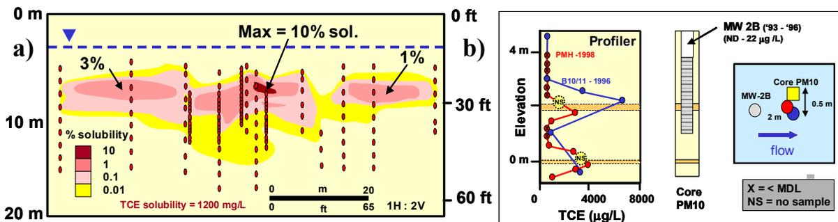
**Figure 1. (a) VOC concentration transect from the Florida Site showing internal variability of plume and (b) misleading data from conventional well revealed by depth-discrete sampling which shows peak concentrations were not detected in monitoring well.**
