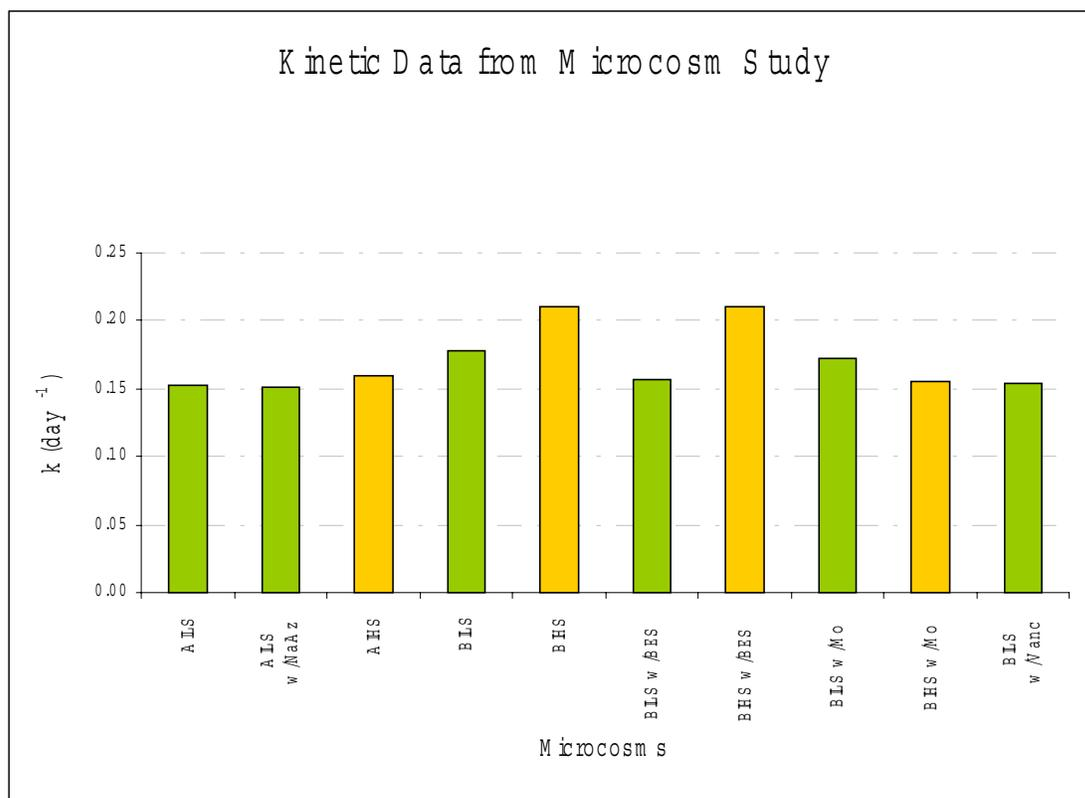
Figure 3 - Kinetic rate for TCE degradation using a batch of microcosms
