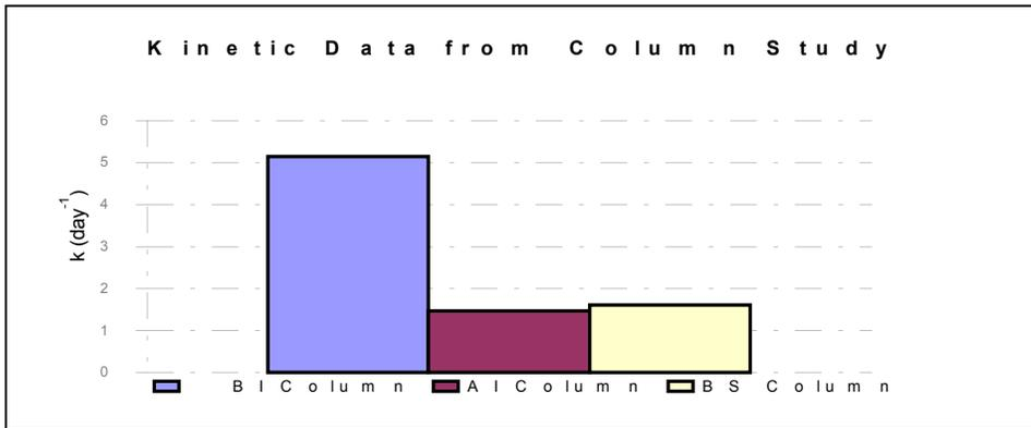
Figure 1 - Rate of TCE degradation in Abiotic Iron, Biotic Iron and Biotic Sand Column
