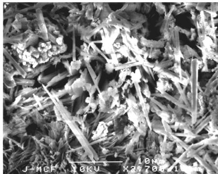
Figure 2 - SEM of deposits on the iron surface in the Biotic Iron Column at 2700 magnification
