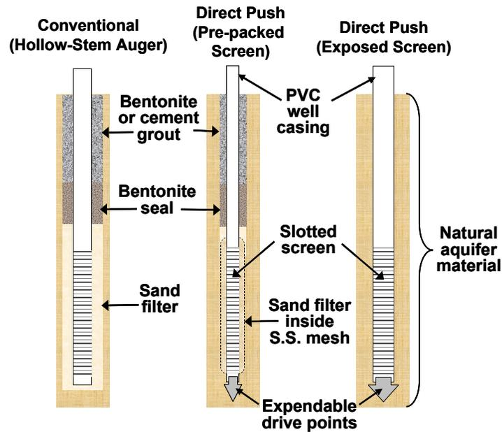
Figure 1 -- DP wells and conventionally drilled well types evaluated using LTM
