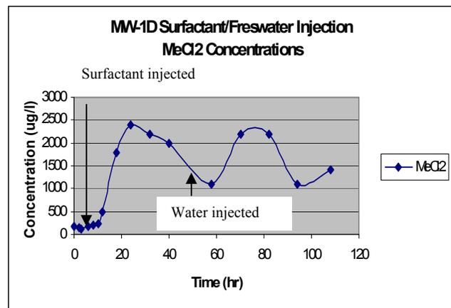
Figure 5: Methylene Chloride breakthrough in MW-1D at Spartan Chemical
