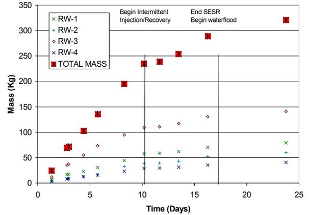
Figure 2: Cumulative TCE and TCA mass recovery (kg) from effluent during surfactant flooding at Alameda Point
