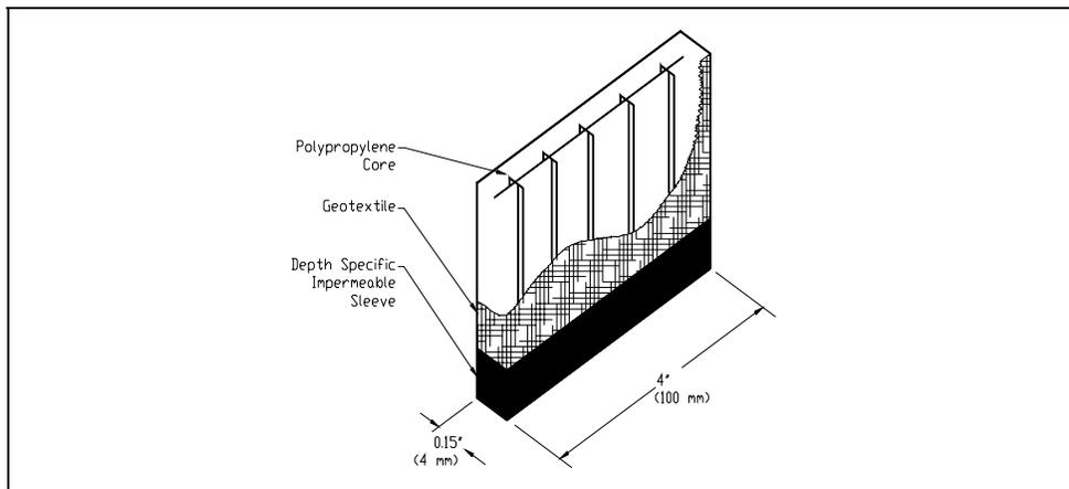
Figure 1 - Prefabricated Vertical Drain
