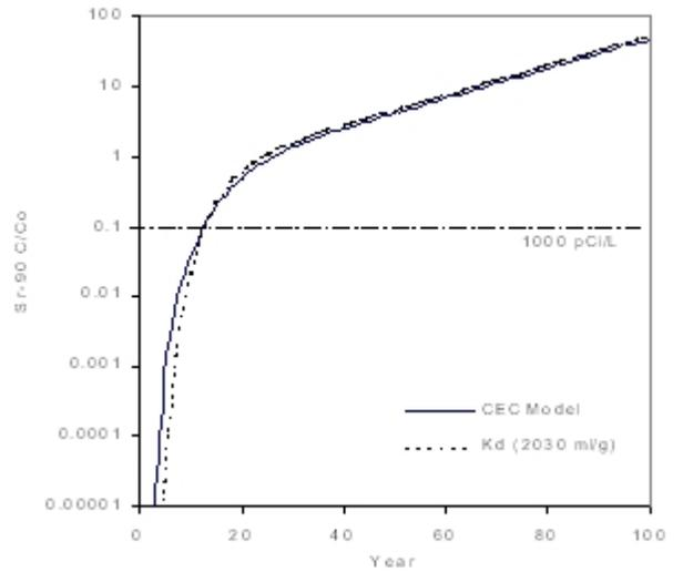
Fig 3. Comparison of modeling approaches for barrier life
