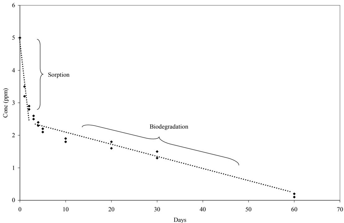
Figure 1: Primary mechanisms of PCE attenuation at OU4 Site.
