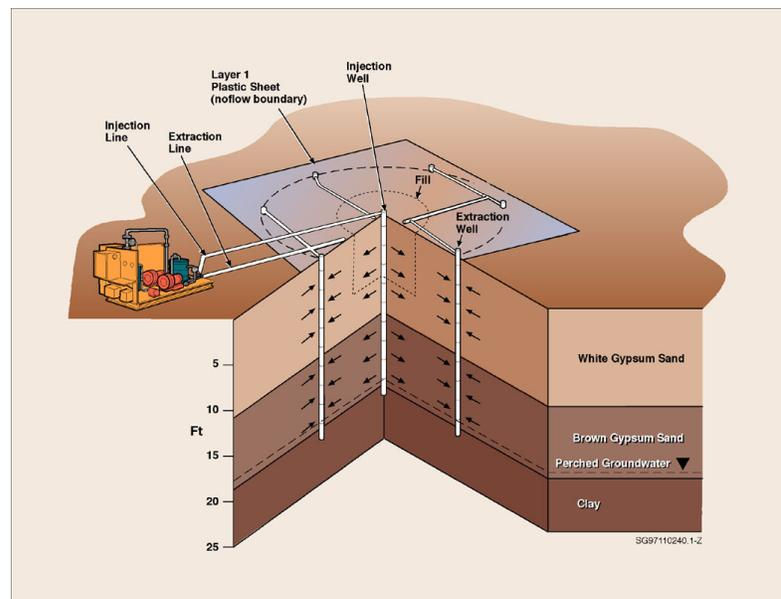
Figure 1. Cross Section of the In Situ Gaseous Reduction Well-Field Network.
