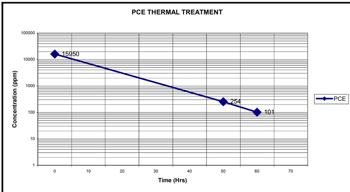
Figure 1: Reduction of PCE through mechanically enhanced thermal desorption over time on a semi-log relationship
