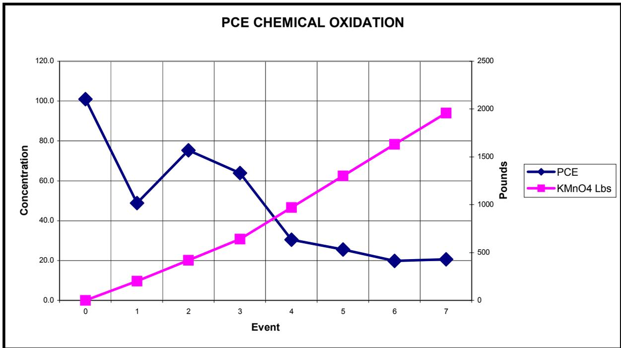
Figure 2: Chemical oxidation of PCE by direct mixing of potassium permanganate with the MITU
