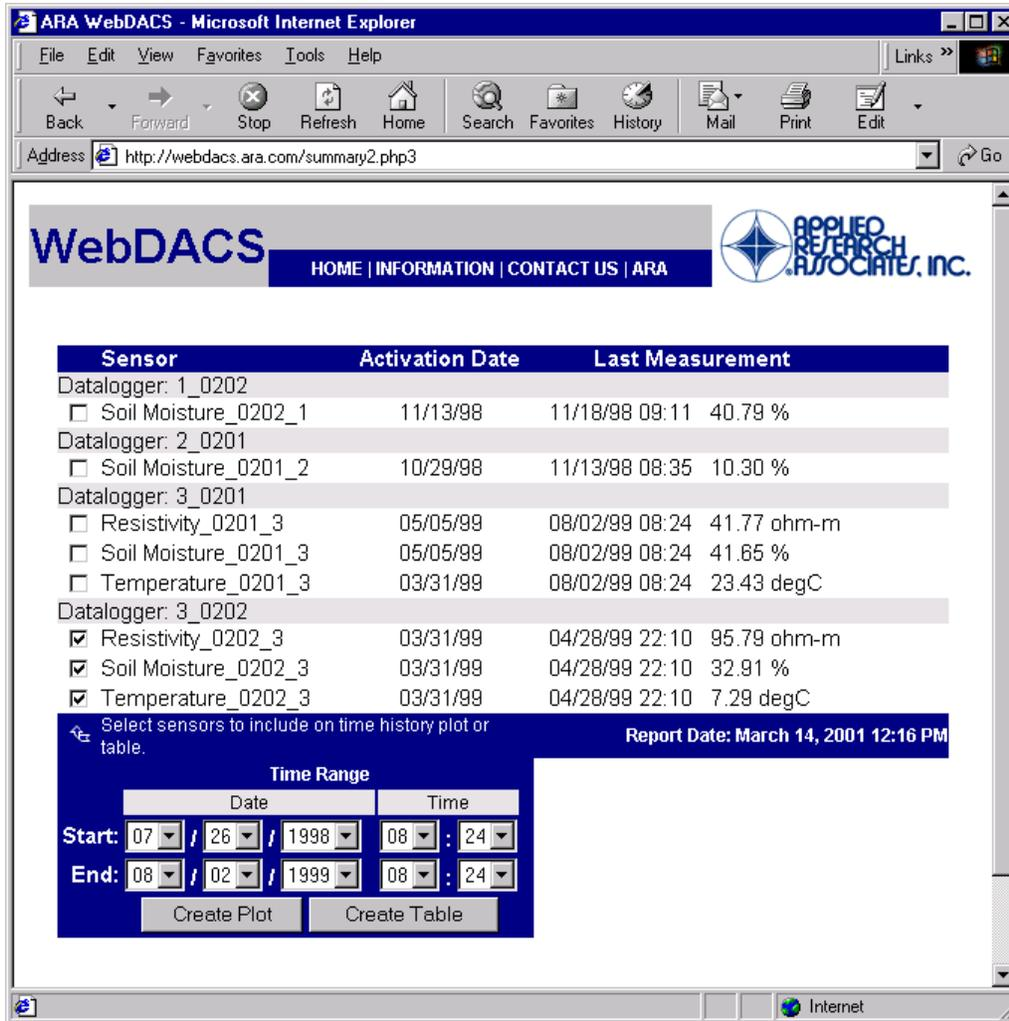
Figure 1. Screen shot of WebDACS sensor summary page. Text entry fields and buttons at the bottom of the page allow the user to generate a plot or tabulation of data from specific sensors selected above over a specified time interval.
